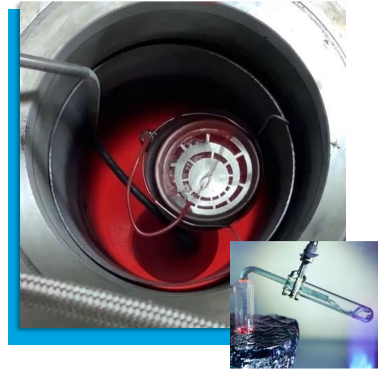
Liquid Fluoride Salt Coolant Flibe ( 2\text{LiF}-\text{BeF}_2 )
