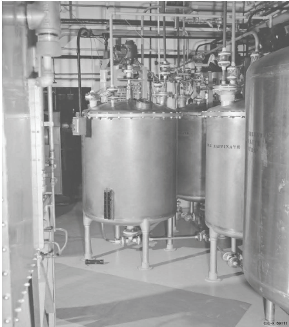
Figure 12. Vessel in which the 1958 Los Alamos process criticality accident occurred.
