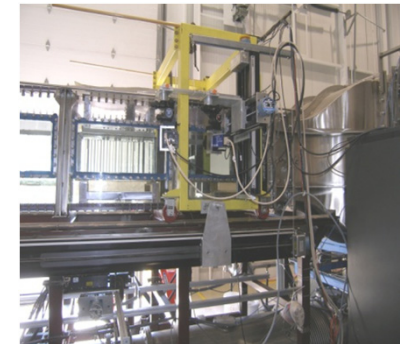
INL's Matched Index of Refraction (MIR) Facility to Study 3-D Flow Effects in Plena
