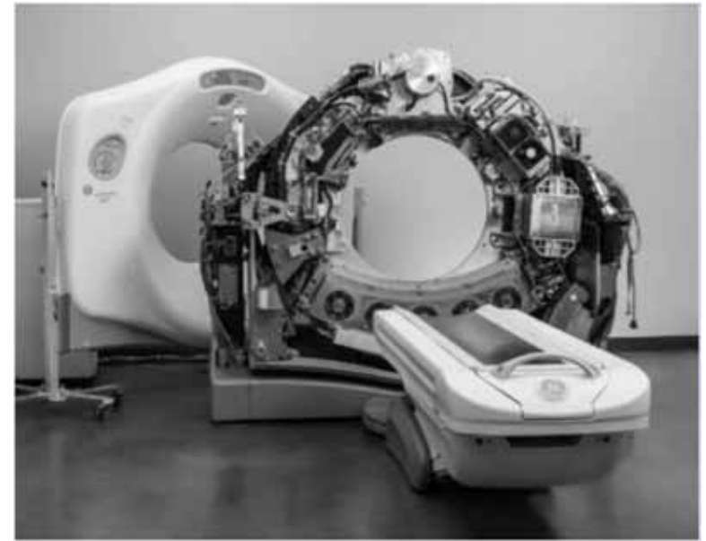
Typical gantry of a conventional CT system with covers removed (photograph of GE Light Speed VCT®).
